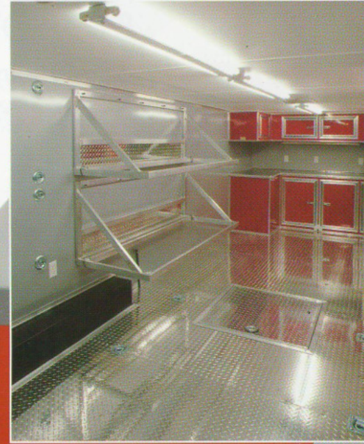
Custom interior featuring wall mounted tire racks, floor and wall mounted D-rings, under floor storage, custom lighting and overhead and workbench cabinetry with optional color panel inserts.
