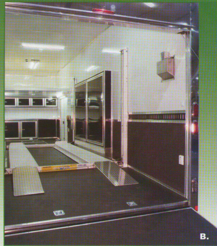
A. Lift system shown in the raised position. B. Lift system shown in the loading position.
